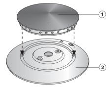
Place the burner cap, ①, onto the burner base, ②, so that the notches fit into the holes (see arrows).
